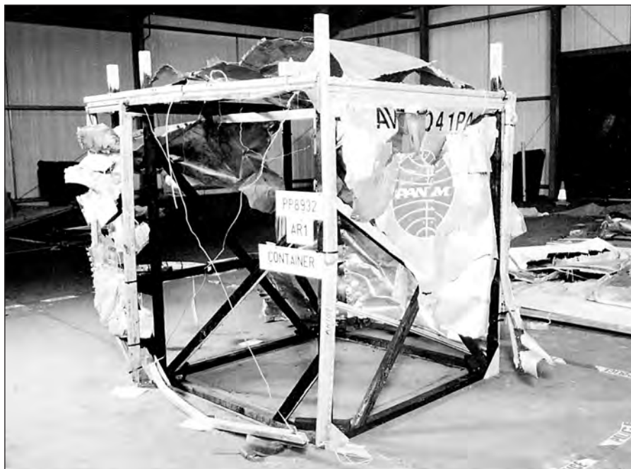
The reconstructed baggage container which went in the hold of Pan Am 103 with the bomb suitcase
